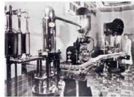
Fig. 10 Postcard of "The Kraft Mayonnaise Kitchen—The Bottling, Jar Capping, and Labeling Machine," Century of Progress International Exposition, Chicago, 1933-34
